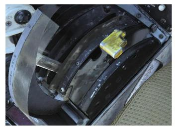
5.b When HZ TAIL AUTH caution light goes out and the OVER flag appears, it takes about 8 seconds, only then you will be able to move EMERGENCY WING SWEEP handle full aft (75° sweep position) and stow (left click on the handle).
