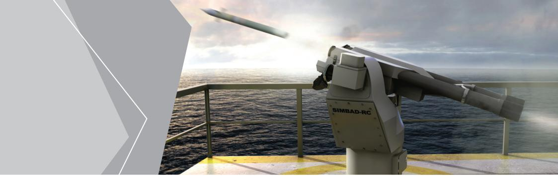
SIMBAD-RC is an anti-air self defence system operating the very effective fire-and-forget MISTRAL missile. It is capable of providing the primary self defence capability for all warships or of complementing the main air defences of first rank warships.
