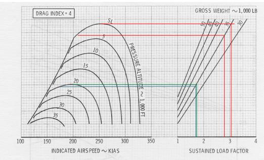
Interesting that the maximum speed obtained from the chart for DI=0 (357 knots) differs from the value obtained from the special chart for maximum speed (345 knots)
