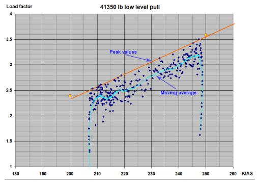
The yellow triangles are the reference points derived from the instantaneous turn performance chart (See Appendix). It's clearly seen that the peaks of load factor matches the reference, but the load factor itself is very uneven, and it's average value is ~10% less giving ~10% loss in turn rate.
