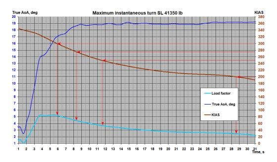
As instantaneous turn rate is only a matter of maximum lift coefficient, sustained turn rate depends on drag polar and available thrust. Very often these polars can be easily derived from the required sustain turn rate but in the case of A-10 the actual drag polars were available, so the task was to compare measured turn rate to the reference values derived from the performance charts.
