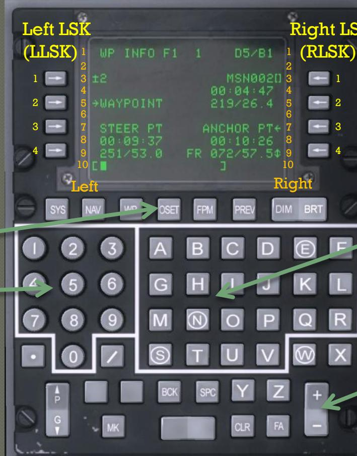
The keys with the arrows on them, that are on both the left and right sides of the CDU are called Line Select Keys or LSK's. They are numbered 1-4 in a descending order.
