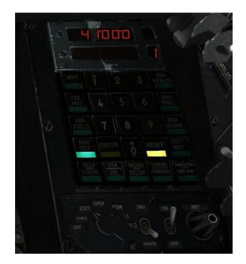
3) Press '0' again to enter positive east coordinates and continue by entering the East coordinate. After the line is full, the enter button will light up, indicating that what you've just entered is recognized and complete.
