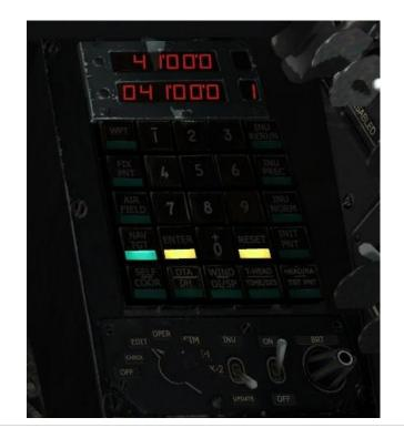
4) Hit enter and go back to normal operation mode and select your new TGT point. It is automatically in the ingress mode.
