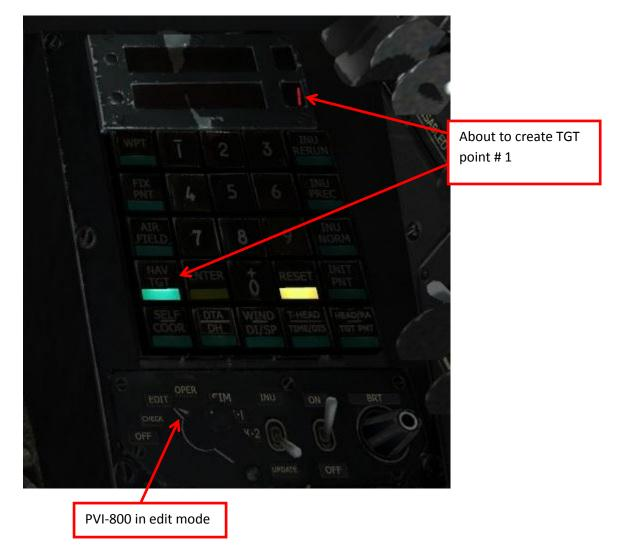
2) Before you enter a coordinate, you will have to determine either positive or negative by pressing '1' (a '-'sign will appear in front of the upper display) or by pressing '0' prior to entering the actual coordinate. All coordinates in this region are positive, so you begin by pressing '0' and then continue to enter the rest of the North coordinate. It will appear in the upper display as you can see in the picture below.
