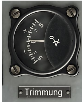
Figure 72: Horizontal Stabilizer Trim Indicator
