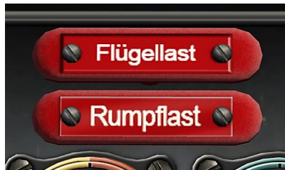
Figure 56: Emergency Fuselage and Wing Load Release
