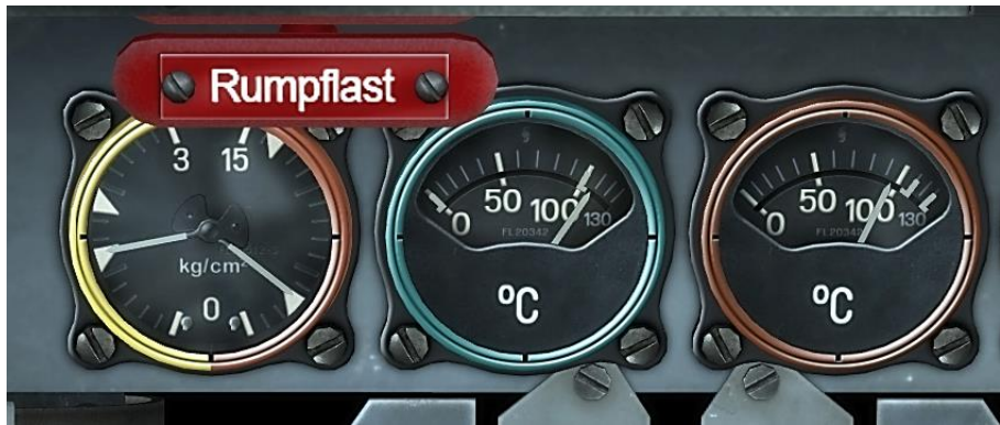
Figure 24: Fuel and Oil Pressure, Coolant Temperature and Oil Temperature Gauges
