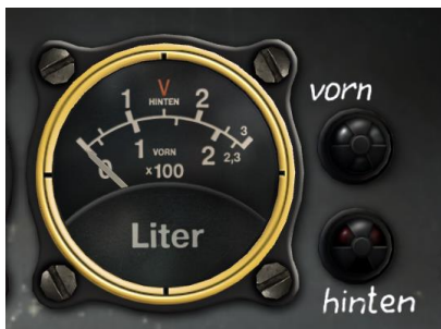
Figure 61: Fuel Contents Gauge with Fuel Warning Lights
