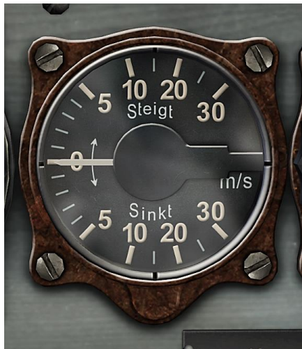
Figure 48: Vertical Speed Indicator
