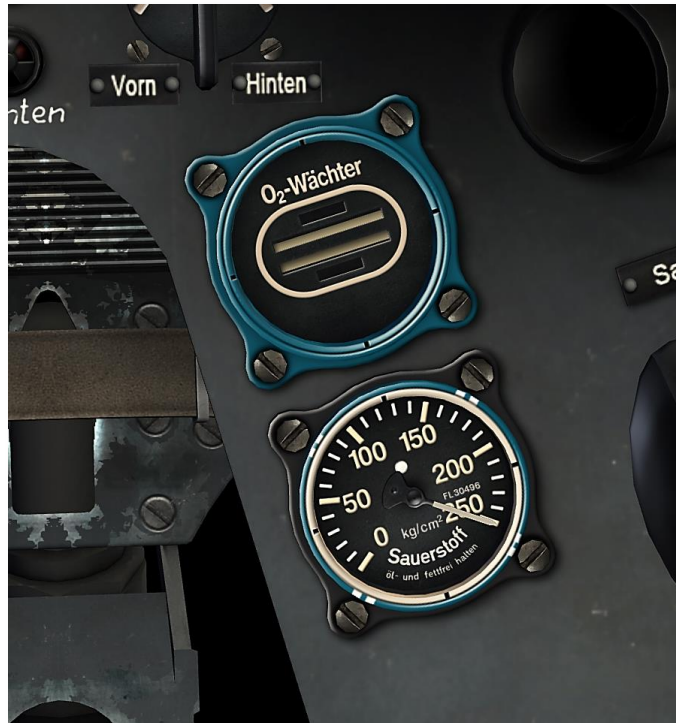
Figure 28: Oxygen Flow Indicator and Pressure Gauge
