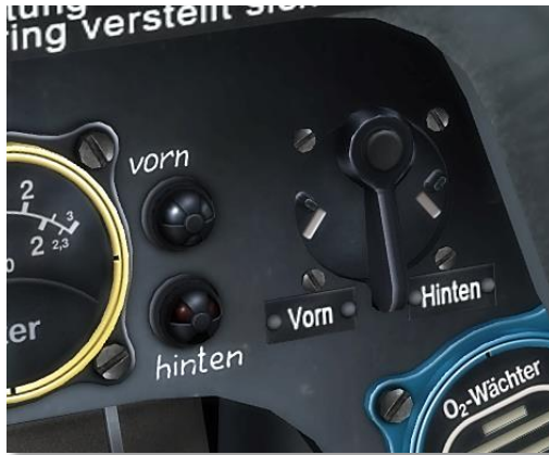
Figure 22: Fuel Warning Lights, and Fuel Gauge Selector Switch
