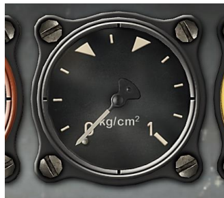
Figure 60: Water/Methanol Pressure Gauge
