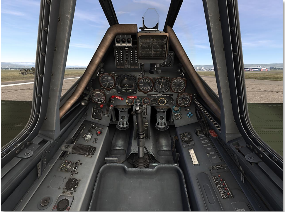
Figure 35: Fw 190 D-9 Cockpit Overview
