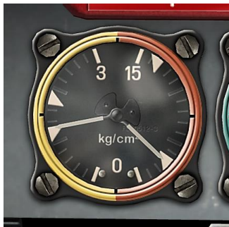
Figure 57: Fuel and Oil Pressure Gauge
