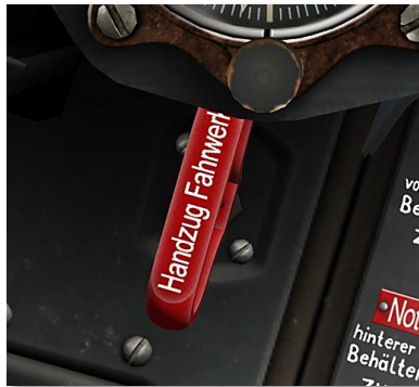
Figure 54: Landing Gear Manual Release
