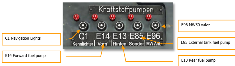
Figure 79: Circuit breakers of additional panel
