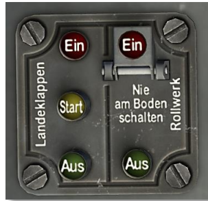
Figure 73: Landing Gear and Flaps Controls
