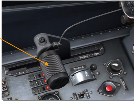
Figure 42: Throttle lever with twist grip and cable
