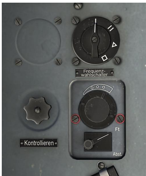
Figure 31: FuG 16ZY Frequency Selector, Receiver Fine Tuning Control, and Volume Control
