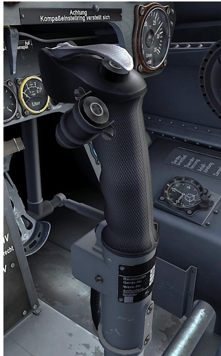
Figure 34: Flight Stick, Trigger, and Bomb Release Button
