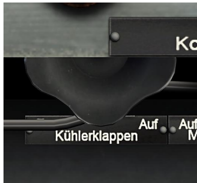
Figure 53: Manual Radiator Flap Control
