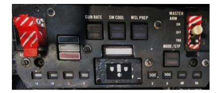
9. EMERG STORES JETT pushbutton light — Out. The MASTER CAUTION light and the EMERG JETT caution light illuminate when the EMERG STORES JETT pushbutton is activated (not implemented on Sim)
