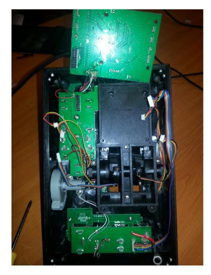
4. After you remove the old/faulty main PCB, proceed to replacing it with the new one, and follow the steps backwards, from no.3 > no.1, as described in this procedure.
