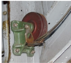
Fig. 16. Gang of rollers in tail boom
