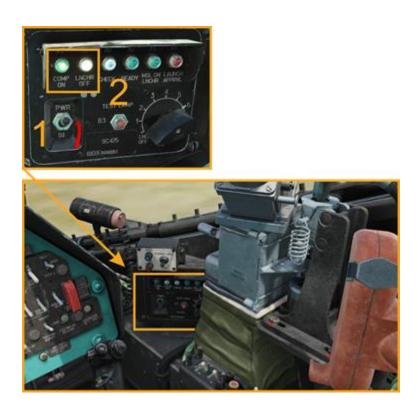
Turn on ATGM sight power (1) and guidance unit panel. The  $\Pi 3$  "L3" light should illuminate:
