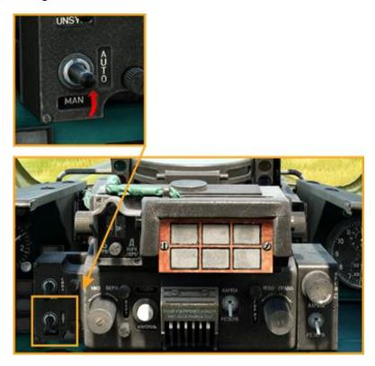
Switch ON the Main Weapon Safety switch in the Pilot-Operator seat (forward cockpit) or use the "Prepare weapons systems" command [LCtrl + W] to ask Petrovich AI to turn on all weapons-related switches in the forward cockpit:
