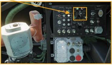
On the right-hand instrument panel of the Pilot-Operator cockpit, turn on the Missile Power switch:
