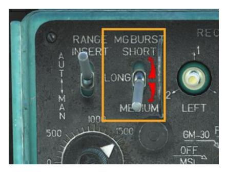
If using the MG30 main cannon, select a desired firing rate:
