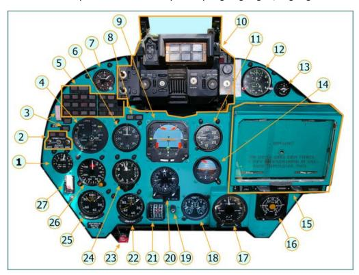
Figure 11. Pilot-Commander Instrument Panel
