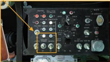
When the OBSERV targeting gyros switch is turned on, the ATGM sight doors will open:
