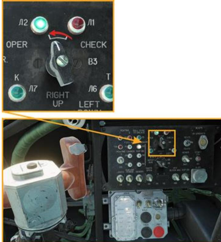
On the right-hand instrument panel of the Pilot-Operator cockpit, turn on the Missile Power switch:
