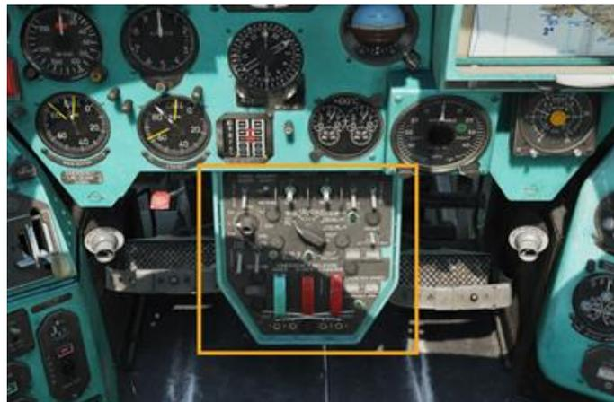
Turn on Aux Stores Lights switch (to enable arm and pylon lights):
