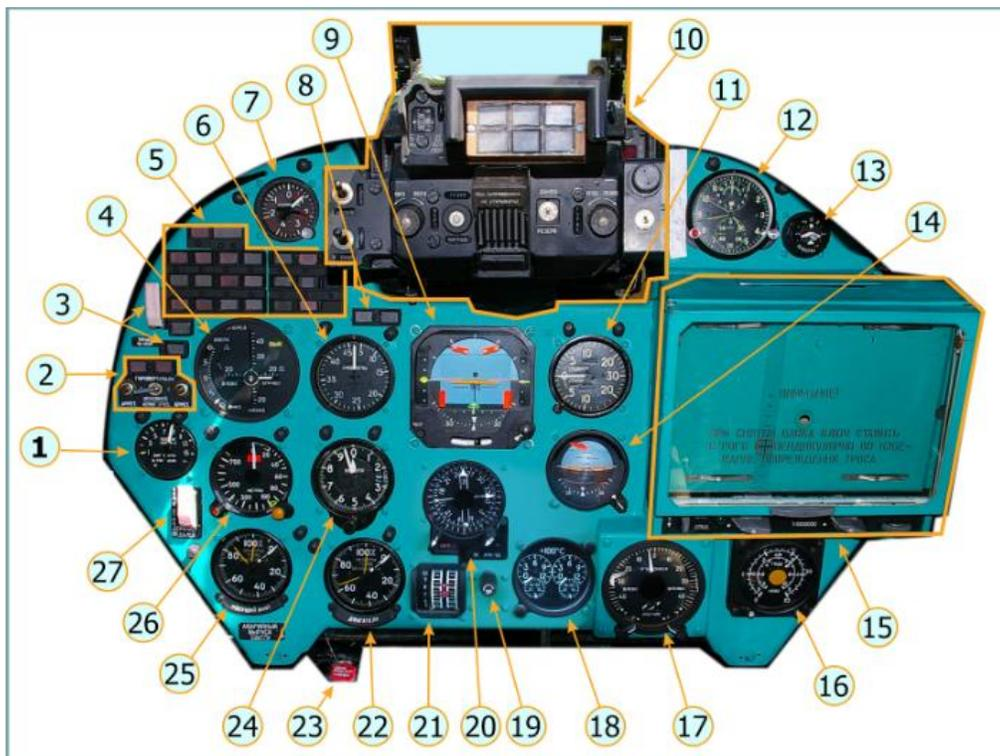
Figure 11. Pilot-Commander Instrument Panel
