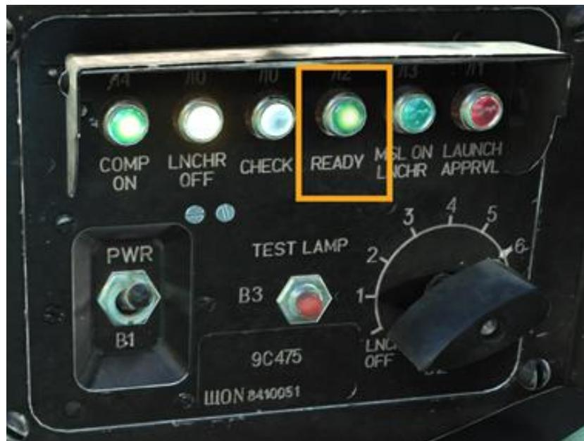
Turn on the OBSERV targeting gyros switch on the guidance unit panel. The Л3 "L3" light will start blinking, and the L4 light will illuminate in 10–15 seconds, indicating that the ATGM sight now can be moved:
