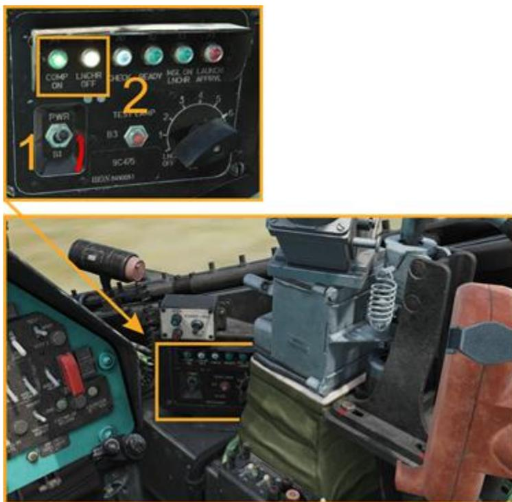
Turn on ATGM sight power (1) and guidance unit panel. The Л3 "L3" light should illuminate:
