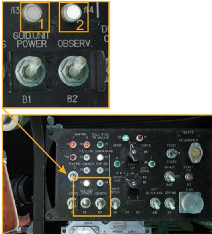
When the OBSERV targeting gyros switch is turned on, the ATGM sight doors will open:
