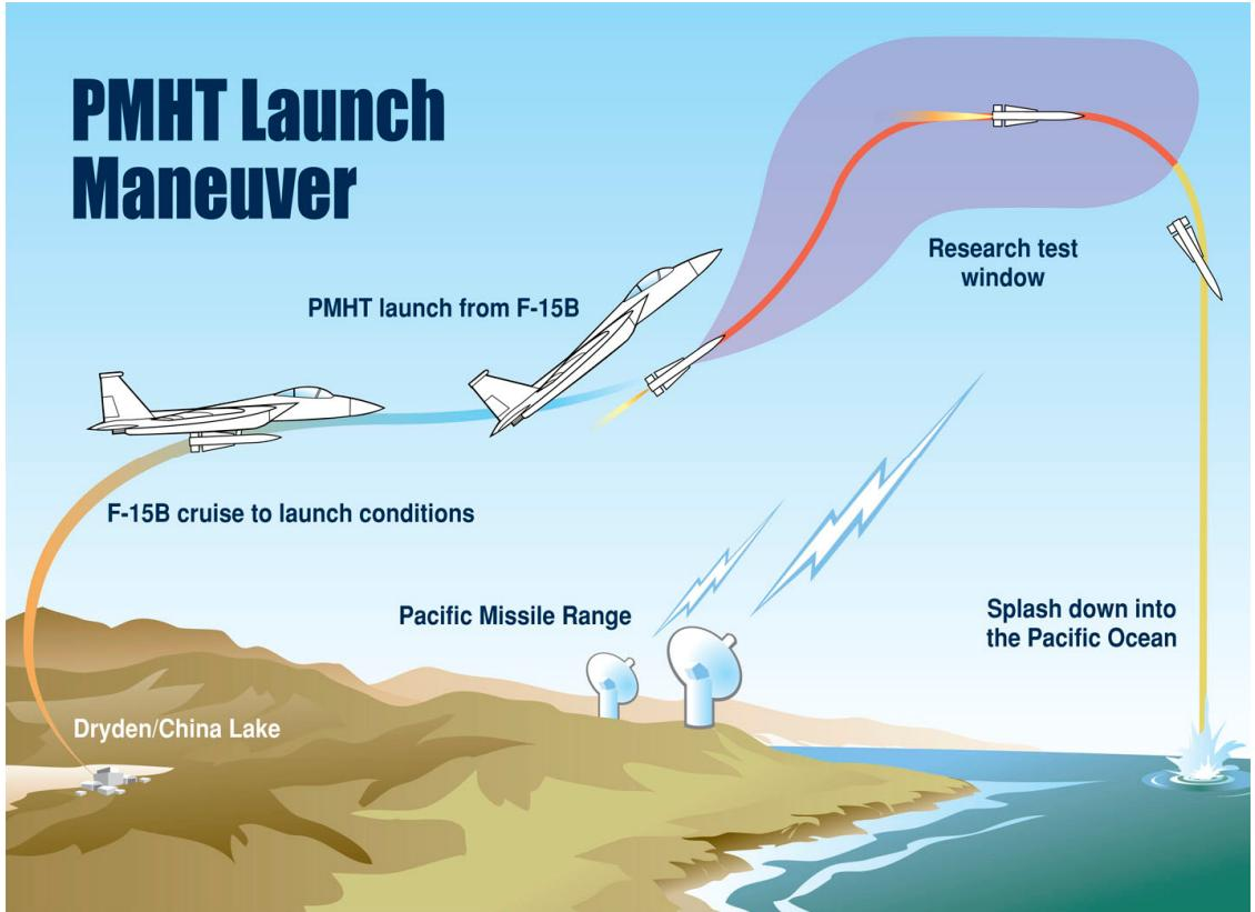
PMHT would be air-launched from NASA F-15B using F-14 launch hardware from within F-15B flight envelope and internally guided to test condition
