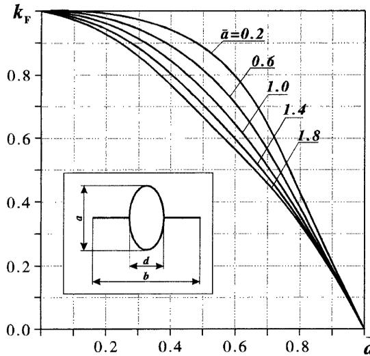
Fig. 3. Cross section shape factor for the elliptical fuselages.
