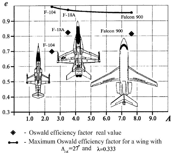
Fig. 1. Influence of the fuselage on the airplane Oswald efficiency factor.
