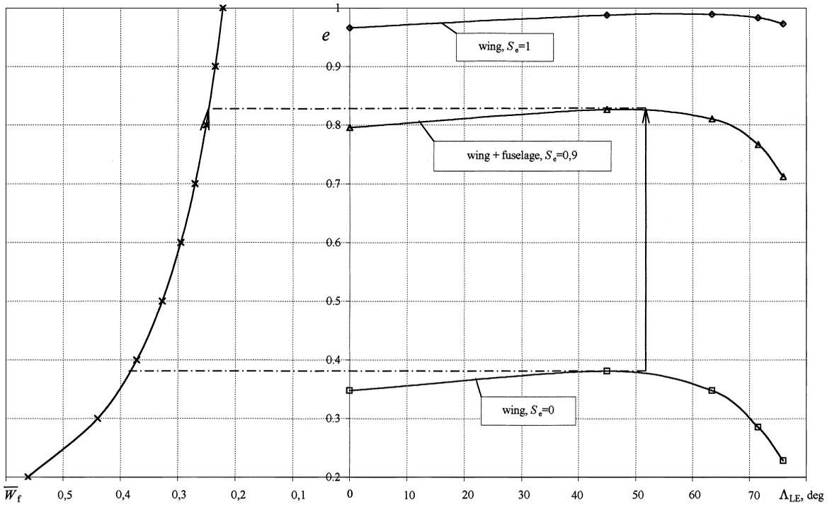
Fig. 2. Effect of the leading edge suction force on a relative fuel capacity.
