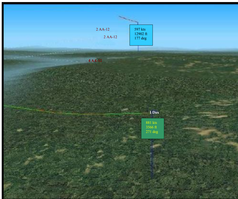
Figure 1c: The Beam is established and maintained at this point, maintaining a heading roughly 270 degrees off from original at full/AB. Missiles are effectively beaten and need only be outrun at this point prior to reengagement is required. This is done by observing its relative motion.
