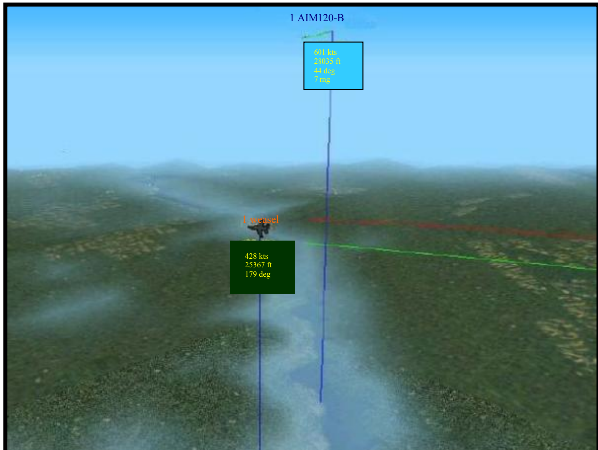
Figure 3b: The initial Offset is seen here, after launch, establishing a left offset roughly 50 degrees left of original course (180). Once wings level, the pilot will immediately go to visual scanning for the AA-12 (in this example a AIM-120 is being used as the hostile missile), also shown here. Music and Radar off, as the remainder of the maneuver is strictly visual, until reengagement.
